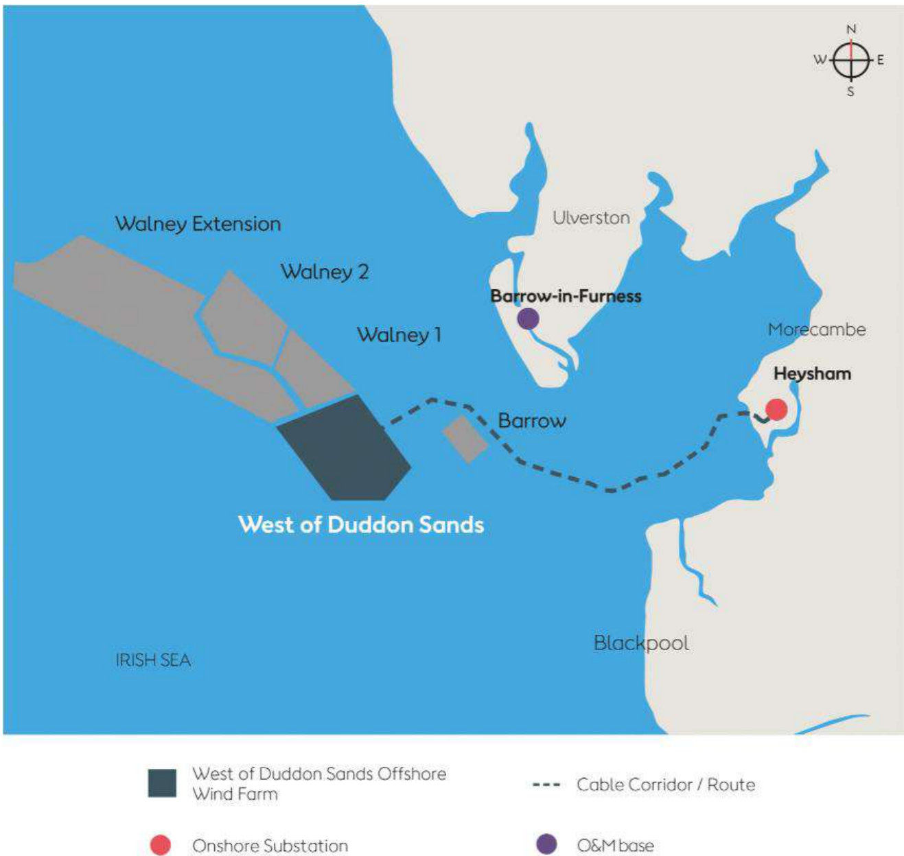
Figure 2.4.17: West of Duddon Sands (2014) Offshore Windfarm Location
