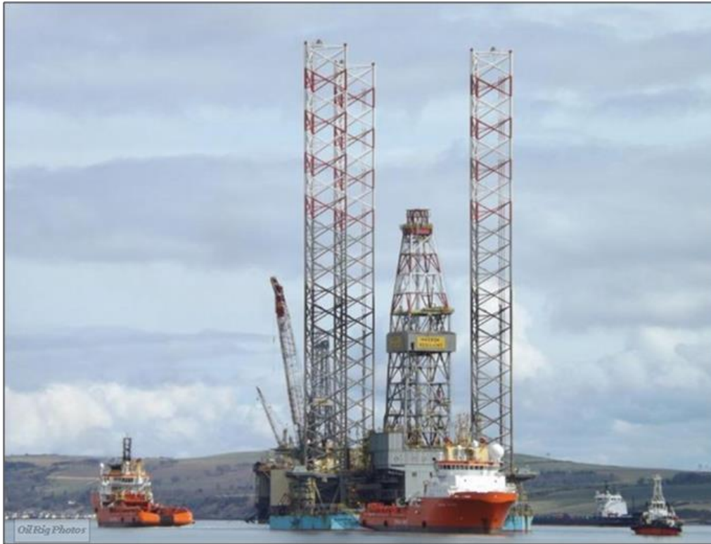
Figure 2-2 Typical Jack-Up Rig Under Tow.
